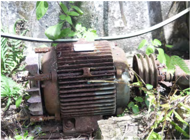
昂坪茶園工場內由意大利電氣製造公司「ERCOLE Marelli & C-S.p.A.」所製的三相電感應電動機。 A 3-phase induction motor - made by ERCOLE Marelli & C-S.p.A., an Italian manufacturer for electrical products - in the tea factory at Ngong Ping tea plantation.
