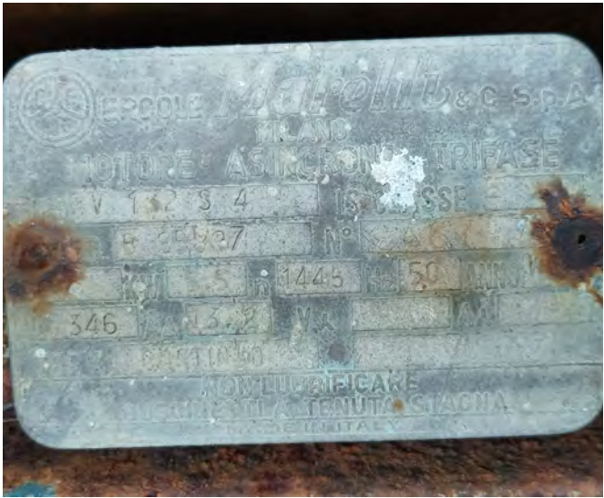
三相電感應電動機的具體資料。 The specifications of the 3-phase induction motor.
